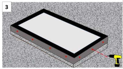
Pre drill fixing holes through aluminium and timber upstand/kerb at 100mm from each corner then at regular intervals.
