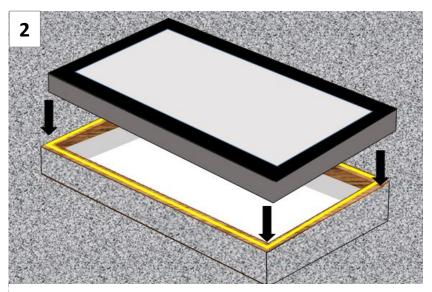
Position the flat aluminium rooflight frame over the top and the side of the upstand/kerb.
