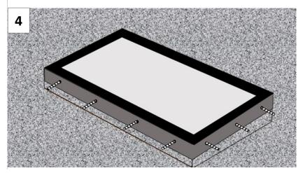
Secure fixing screws with horse shoe packers and finishing caps continuously all the way around securing the aluminium frame in place.
